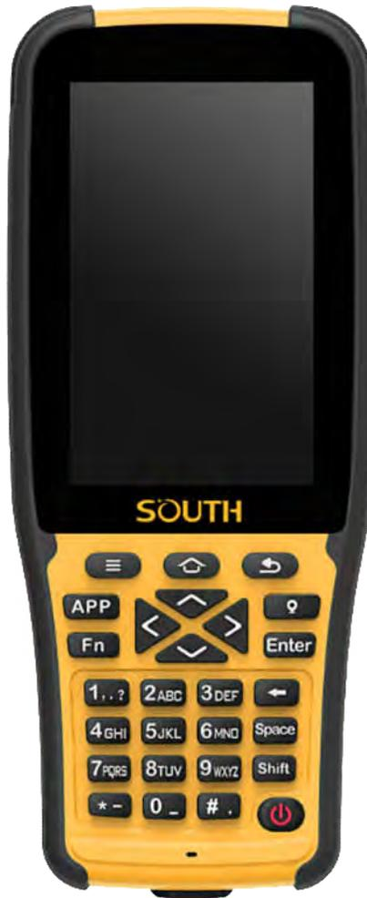
H5 is a new generation professional controller running on Android which offers state of the art smartphone capabilities combined with rugged professional quality. And the alphanumeric keypad which gives flexibility for surveyors' field work.
