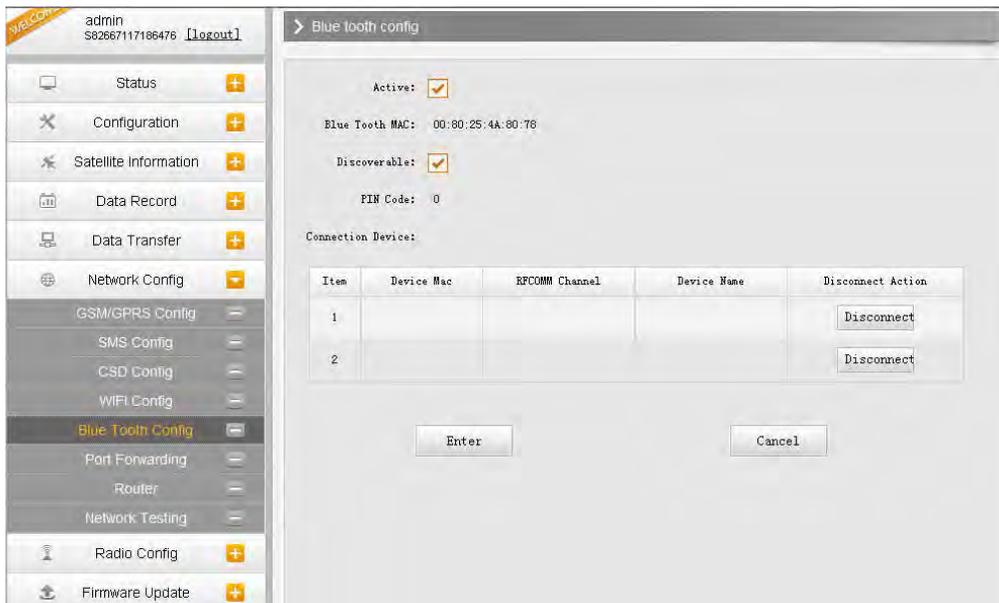
The screenshot shows the 'Blue tooth config' page. The left sidebar contains a menu with options like Status, Configuration, Satellite Information, Data Record, Data Transfer, Network Config, GSM/GPRS Config, SMS Config, CSD Config, WiFi Config, Blue Tooth Config (highlighted), Port Forwarding, Router, Network Testing, Radio Config, and Firmware Update. The main content area displays the following configuration:
