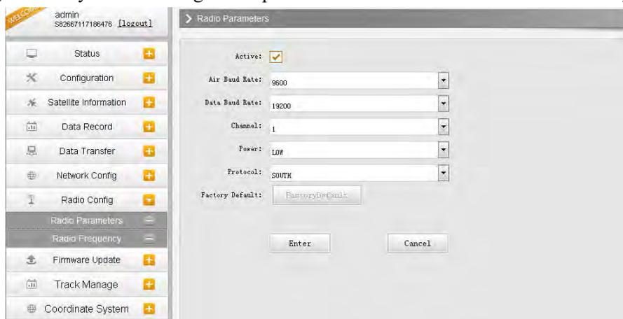
**Air Baud Rate:** This represents the data transmission rate in the air of internal radio, the higher value, the bigger of data size transmitted per second, usually keep the default setting.
